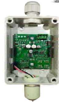
Probe with sensor remounted
