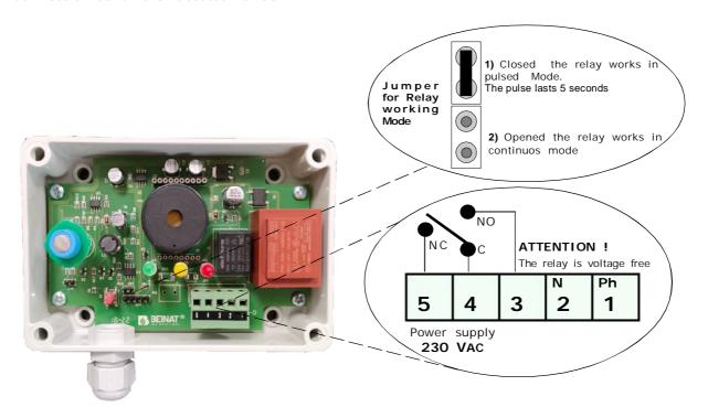
Diagram of connection with a valve normally open 230VAC
