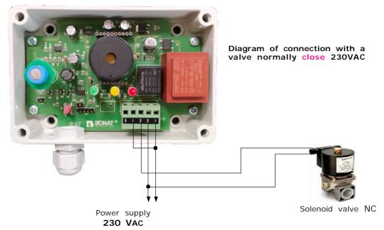
One or more detectors with a valve normally closed 230VAC
