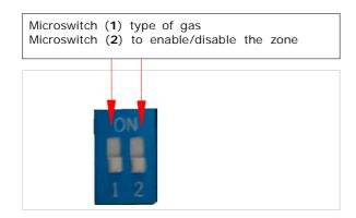
Switch 1 - To select the type of gas to be detected ON position, you get reading in L.E.L. Explosive gases OFF position, you get reading in ppm. Toxic gases Switch 2 - To enable or to disable the zone ON position, you enable the zone OFF position, you disable the zone
