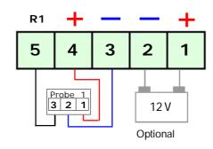
Connections of a solenoid valve Normally Closed without Positive Safety
