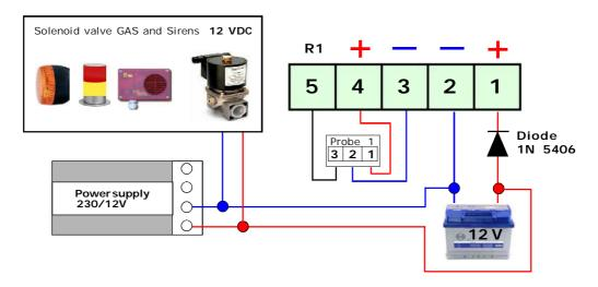
Connections to Positive Safety disabled and an external power supply for valve control and siren 12 V DC  $\,$
