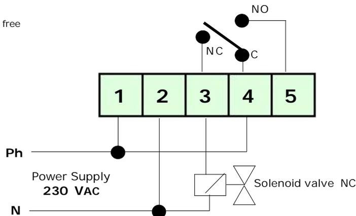
**Diagram of connection with a valve normally open 230VAC**
