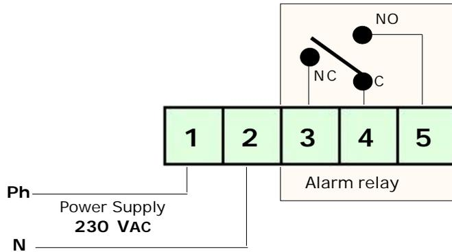
**Diagram of connection with a valve normally close 230VAC**
