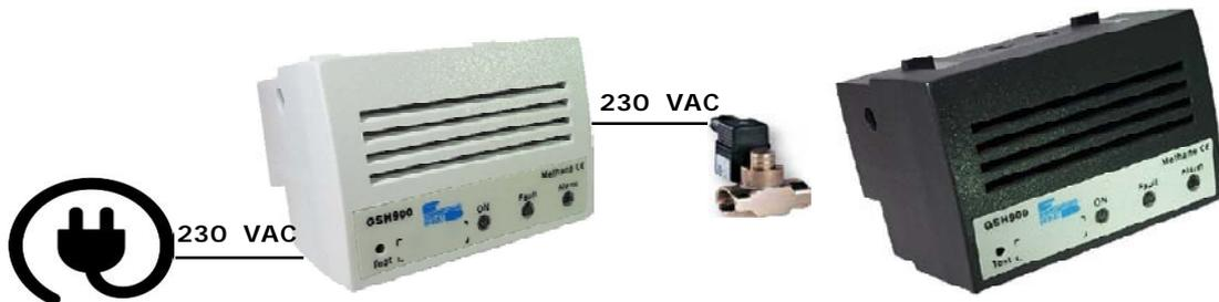
Using the catalytic sensor, the **GSH900** detector detects the presence of **explosive gas** such as: Methane and LPG, with trip sensitivity calibrated at 10% of L.E.L. According to the **CEI 216- 8 Norm of 2005**, the detectors are triggered by a specific combustible gas concentration in the environment. The detectors should tolerate common vapours and interfering substances usually present in household environments, and guarantee a high stability with temperature and humidity variations.
