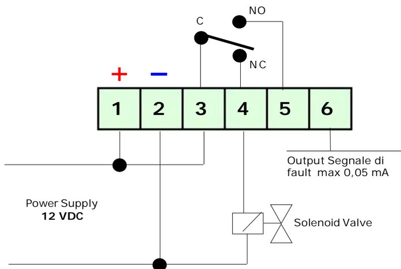
**One or detector with 12V normally open valve**
