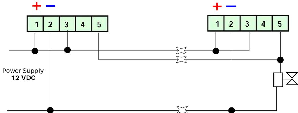
**One or more detectors with 12VDC normally closed valve**
