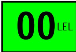
The green display shows an absence of leakage of gas, normal conditione
