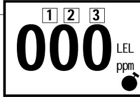
A row of LEDs numbered from **1 to 3** and called PROBES has been fitted on the **GS300-Mc**. These LEDs are lit with a 4 second frequency representing the connected probes, and indicate the probe being read on the display.
