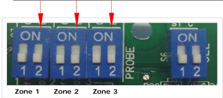
**Relay's working mode and the memory of the Main alarm**
