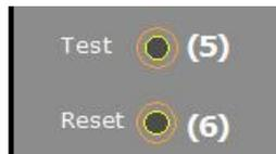
The simultaneous and prolonged pressure for 5 sec of the "TEST" and "RESET" buttons enables the test-on mode in which the control unit does not switch the general alarm relay for a period of 15 minutes; Not even pressing the external manual button.
