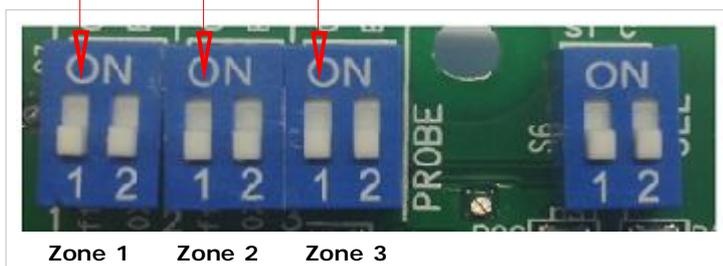
**Selection of the type of gas monitored by each probe**
