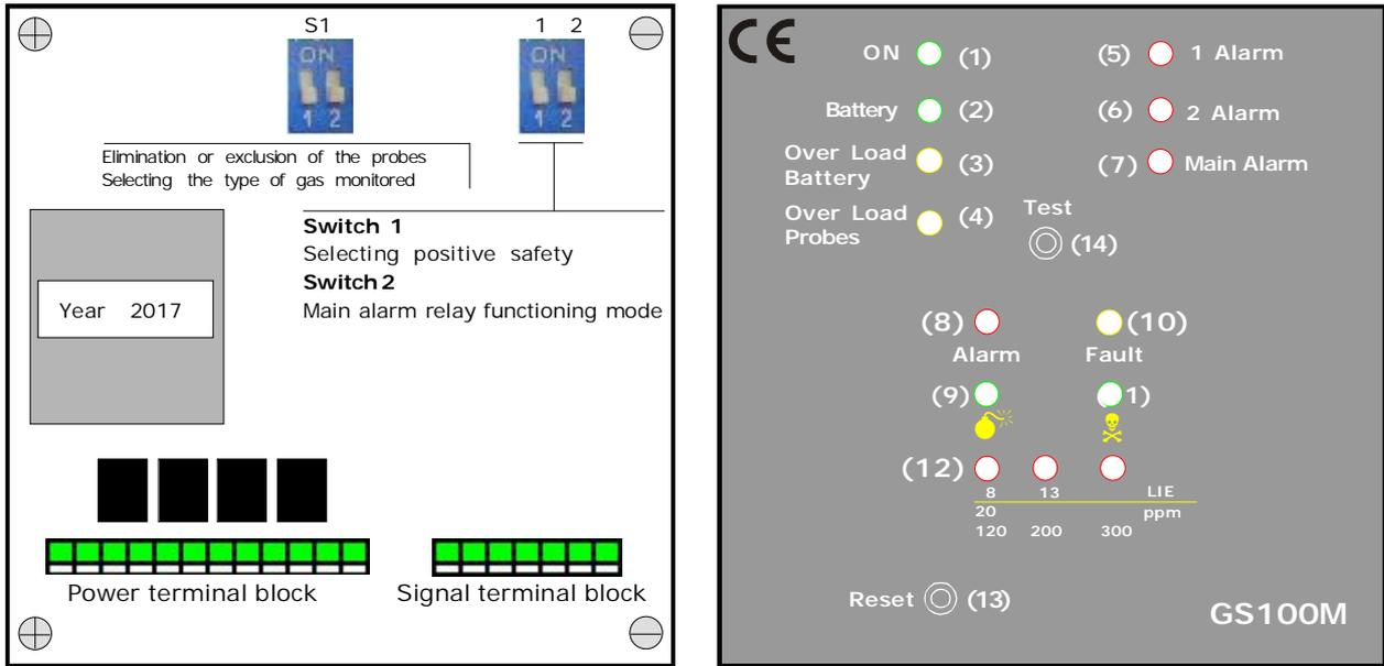
**1) MAINS LED.** It lights up when electrical power is connected. Initially, this LED blinks for about 1 minute waiting for the check.
