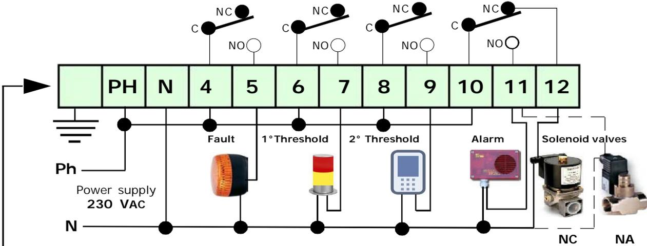
**Connections of a solenoid valve Normally Closed with Positive Safety**
