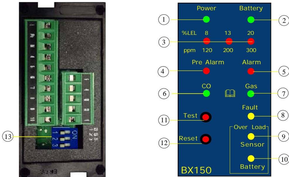
**1) MAINS LED.** It lights up when electrical power is connected. Initially, this LED blinks for about 1 minute and a half waiting for the check.
