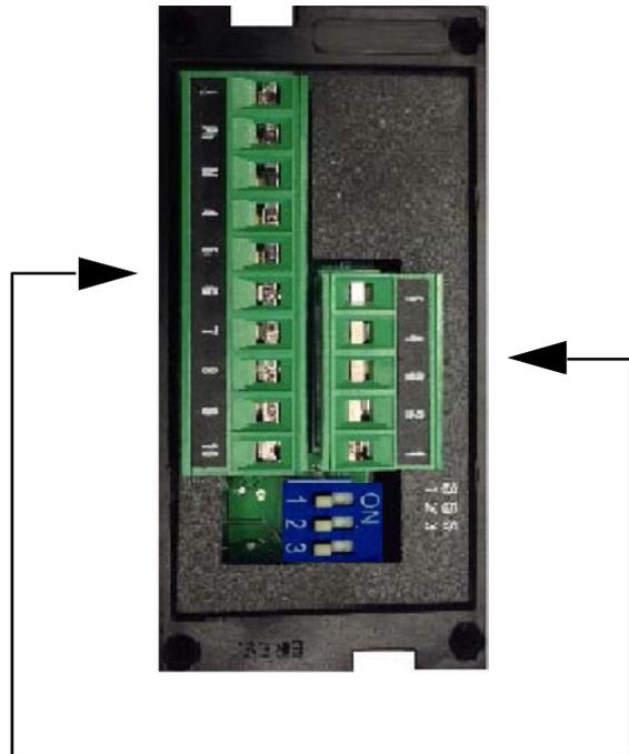
Diagram of the terminal block relay
