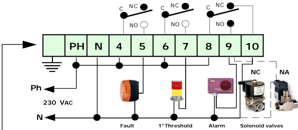
**Connections of one solenoid valve Normally Closed with Positive Safety**
