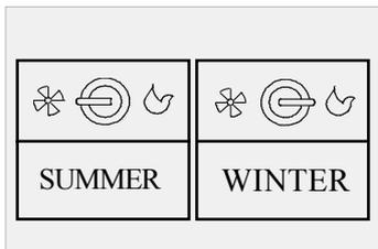
The **LC150** has a switch for selecting the operating mode. Placing the switch as in the first drawing to the left, the thermostat work in SUMMER mode, vice versa, as specified in the second drawing on the right, the thermostat is operating in WINTER.
