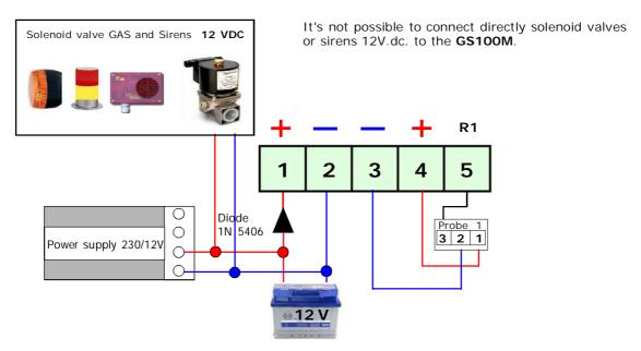
Connections with Positive Safety disabled and an external power supply for solenoid valve and siren control to 12 VDC
