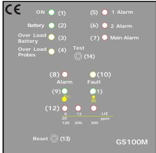
1) MAINS LED. It lights up when electrical power is connected. Initially, this LED blinks for about 1 minute waiting for the check.
