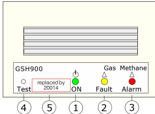
**1) MAINS** connected indication **LED**. After turning on, the **GSH900** performs a test of the sensor's efficiency status, and gets it to the functioning temperature. This phase lasts about 60 seconds. At the end, the detector will issue a **"BEEP"**. Then it is ready for detection.
