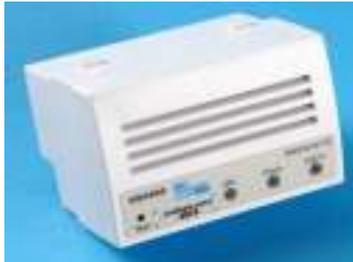
Using the catalytic sensor, the **GSH900** detector detects the presence of **explosive gas** such as: Methane and LPG, with trip sensitivity calibrated at 10% of L.E.L. According to the **CEI 216- 8 Norm of 2005**, the detectors are triggered by a specific combustible gas concentration in the environment.
