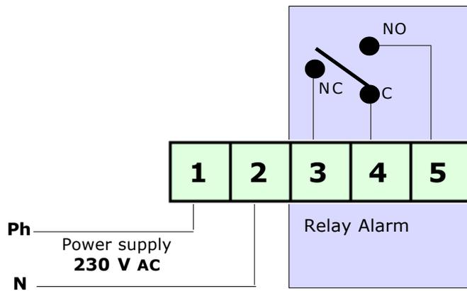
**One detector with 230V AC normally close valve**
