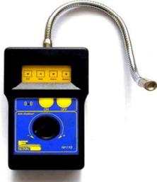
The **RP110** portable gas detector is an electronic instrument manufactured by **BEINAT S.r.l.** to help technicians during testing or to search for and locate leaks in gas heating appliances. The **RP110** detects the presence of:
